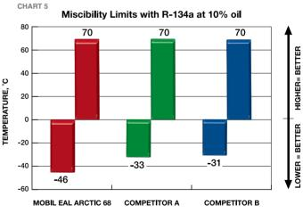
Relative to corresponding competitive products, Mobil EAL Arctic Series provides optimum compatibility over a broad evaporator temperature range for many HFC refrigerants such as R-134a (Chart 5).
