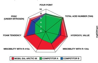
Mobil EAL Arctic 68 demonstrates well-balanced performance on key refrigeration oil parameters. Compared with competitive POE products, it has superior miscibility with key HFC refrigerants such as R-134a and R-410a.
