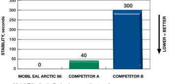
Mobil EAL Arctic Series has excellent performance with respect to foaming tendency (the amount of foam generated, Chart 1) and foam stability (the length of time it takes for the foam to break up, Chart 2), which provides improved equipment lubrication.
