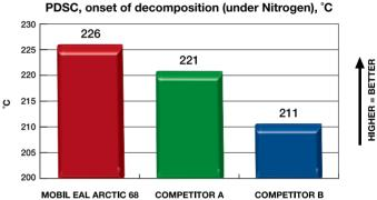
Charts 3 and 4 demonstrate the excellent hydrolytic and thermal stability of Mobil EAL Arctic Series relative to corresponding competitive products. Strong performance on these parameters equates to longer oil service life and improved refrigeration system performance due to improved equipment cleanliness.
